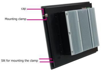
5. The first and second clamps must be positioned and secured diagonally prior to mounting the rest of the clamps. Tighten the clamp's screw using an electric screwdriver by pressing the flat cap onto the back of the panel.
