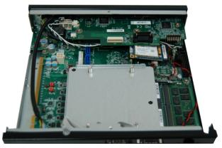
2. Push the Mini PCIe card down and use the provided mounting screw to secure the card on the system board.
